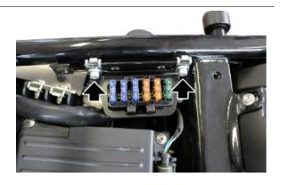
Move the filter box to the side enough to allow removal of the fixing screws (2) on the left side of the filter box support.
