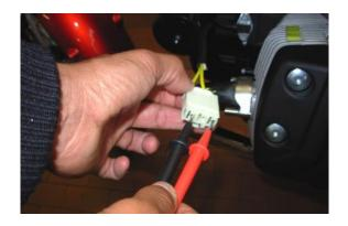
Take the measurement; The correct value is determined by subtracting the wire resistance
