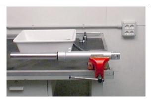
Unscrew the upper closing cap. Pay attention to the possible thrust that the spring can cause to the loosened cap.
