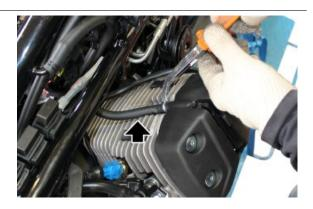
Remove the fixing screws of the injectors and disconnect them
