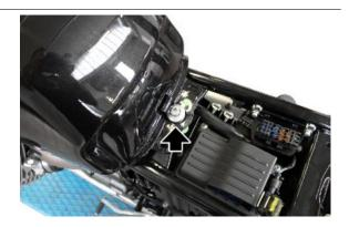
Partially lift the fuel tank in order to be able to disconnect the fuel hose fitting, avoiding damaging it.
