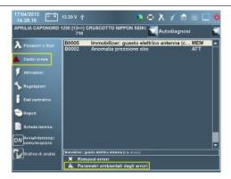
Repeat the operation by selecting each error and showing the corresponding Ambient parameter error (where provided).
