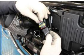
Remove the starter motor to allow the removal of the left lambda probe wiring.
