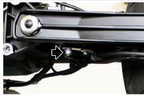
Remove the ABS sensor and the brake calliper
