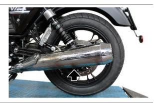
Remove the fixing nut of the cable grommet plate and disconnect it from the swingarm
