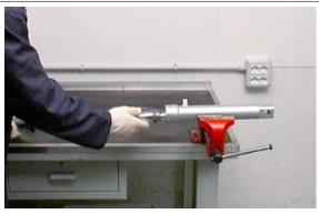
Insert the bearing tube in the wheel holder and push it until it stops.
