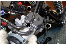
Loosen the gas cables fixing nuts on the throttle body and unhook them
