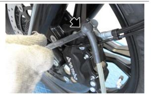
Remove the rubber protection cover from the bleed valve.
