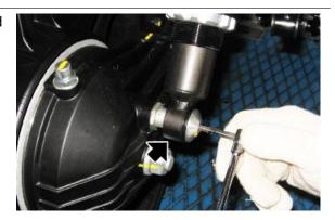
Remove the screw and the relative nut fixing the left rear shock absorber
