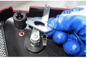
Extract the ignition switch assembly externally
