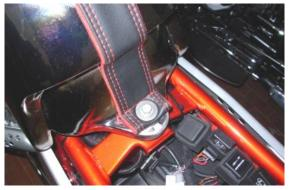
Partially lift the fuel tank in order to be able to disconnect the fuel hose fitting, avoiding damaging it.
