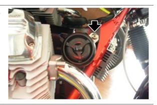
• Unscrew and remove the rear screw.
