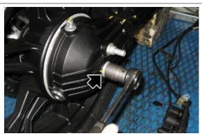
Loosen the wheel pin locking screw.
