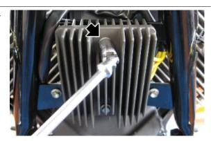
Operating from the left side of the motorcycle, remove the ABS modulator
