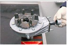
Correctly insert the stud bolts of the gearcase in the holes of the swingarm.
