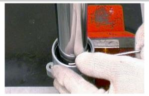
Slide off the bearing tube from the wheel holder fork leg together with the sealing ring, the cap, the upper bushing and lower bushings.
