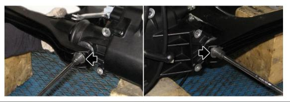
Remove the shimming washer between the swingarm right arm and the gearbox.
