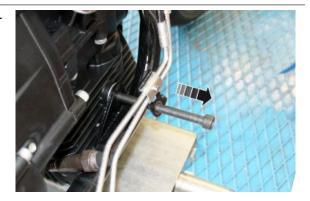
Remove the front fastening screws covers of the cradle
