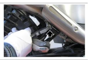
Unscrew and remove the fixing screw of the silencer at the support bracket and recover the nut and the washer.
