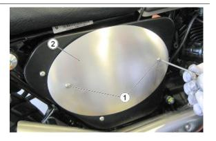
Undo and remove the three fixing screws (3) of the side fairing.
