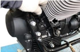
Remove the front screws fixing the cradle, making sure to recover the nuts and washers
