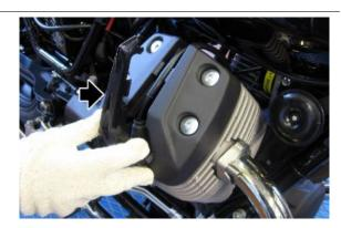
Disconnect the spark plug tube
