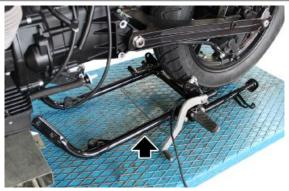
Remove the cable grommet and disconnect the cable harness from the rear brake pipe
