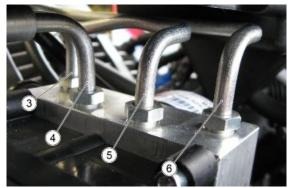
Unscrew the nut of the oil pipe (3) and cover both the pipe and the hole on the modulator.
