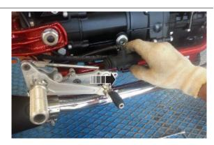
Remove the brake pipe by acting on the fitting and remove the complete pump
