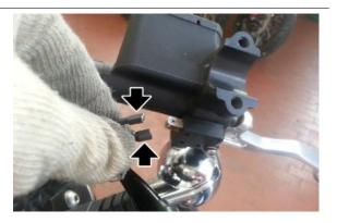
Remove the two brake pump fixing screws
