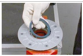
Slide off the bearing from the cover using the suitable punch.
