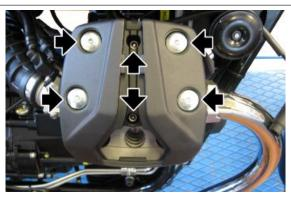
Remove the head cover together with the gasket
