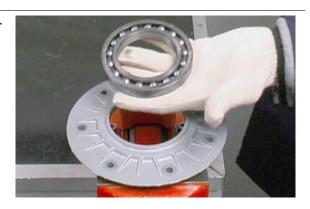
Remove the gaskets unit made up of paper/steel/paper or foamet/steel/foamet
