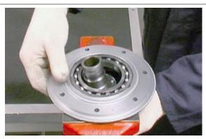
• Remove the sealing ring.
