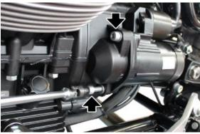
Remove the starter motor
