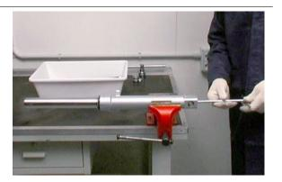
Remove the dust scraper using a screwdriver as a lever.
