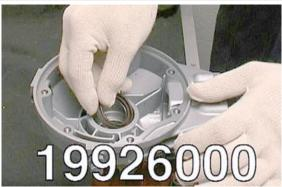
Fit the external ring of the needle bearing on the housing using the suitable punch (19926500).
