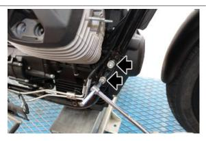
• Remove the two rear screws that fix the cradle
