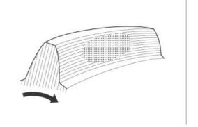
If the contact is like this, the crown is too near the pinion rotation axis: detach the crown by increasing spacer thickness.
