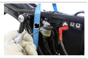
Remove the lower screws of the wheel housing
