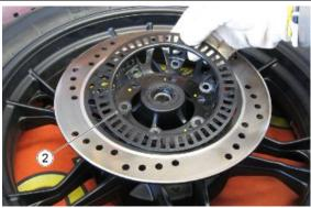
Remove the brake disc (3)
