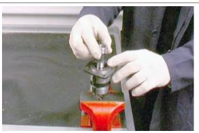
Insert the grooved shank of the pinion on the tool (19907100) and tighten the nut.
