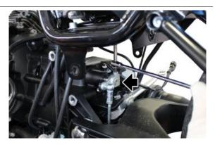
Remove the cradle together with the side stand and gear footrest
