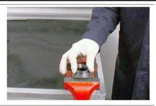
Fit the internal ring of the bearing on the pinion using the suitable punch (19926200).
