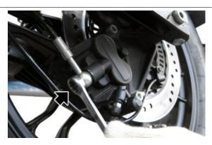
• Remove the two calliper fixing screws
