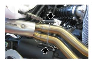
Undo and remove the screw fixing the central muffler to the support bracket.
