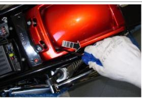
Remove the front screws (2) that secure the mudguard to the frame, taking care to recover the nuts
