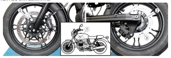
When the sensors (3) detect a significant speed difference between the rear and the front wheels (for example, when rearing up on the back wheel), the ABS system could take this as a dangerous situation. In this case, two things may occur:
