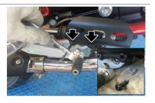
Take the pump from the brake pump shaft
