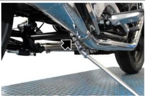
Unscrew and remove silencer retaining nut and collect the screw and the bushing
