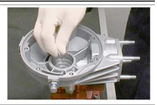
Fit the sealing ring on the housing using the suitable punch (19926000).
