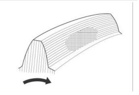
If the contact is like this, the pinion is too near the rotation axis of the crown: detach the pinion by reducing spacer thickness
