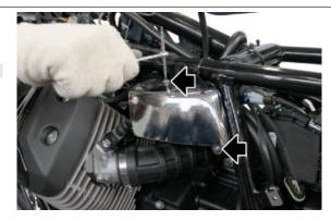
Loosen the clamp between the exhaust end and the catalytic converter
