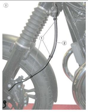
3. Speed sensor wiring harness
