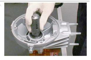
• Fit the bearing on the cover using the suitable punch.
