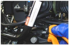
Position the air filter box support, taking car to pass the neutral switch cabling through the hole
