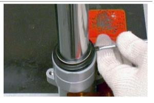
• Slide the dust scraper off and upwards.
