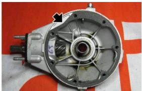
Fit the drilled bolt-crown unit cover and their spacers and gaskets on the housing and provisionally tighten the screws.
