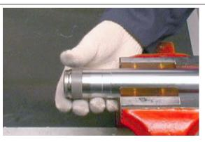
Reassemble the bearing tube in the wheel holder fork leg.
