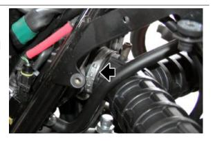
• Loosen the clamps that secure the sleeve to the intake manifolds
