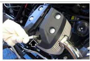
Remove the six head cover fixing screws and collect the washers
