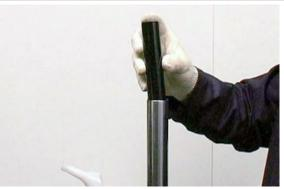
Place the cap on the bearing tube, taking care not to damage the O-ring.
