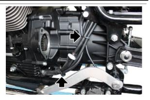
• Disconnect the connectors of the lambda probes
