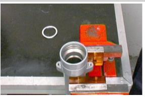
Insert the lower sliding bushing in its seat on the bearing tube.
