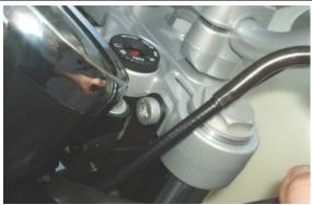
• Unscrew and remove the central nut.
