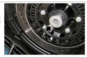
Remove and if necessary replace the six flexible couplings
