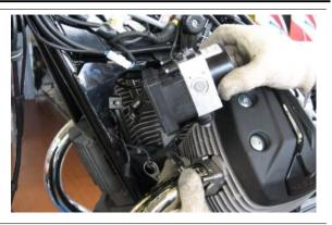
To remove the ABS modulator from the support, remove the three fixing screws
