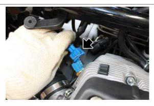
• Loosen the retainer clamps of the sleeve, from the intake pipe
