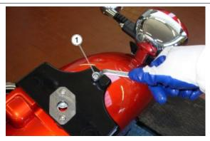
After unhooking the opening cable from the ignition switch assembly, remove it from the mudguard.
