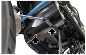
Remove the clamp, remove the wheel housing to allow sliding off the tank
