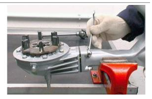
Slide off the gearcase together with the swingarm.
