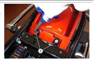
Remove the lateral screws (3) that secure the mudguard and the passenger handgrips from both sides, taking care to recover the nuts
