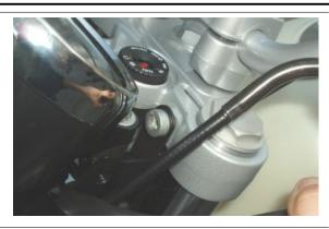
Undo the lower sealing screw.
