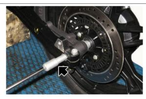
Remove the rear brake calliper support
