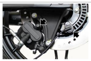
Unscrew and remove the fixing screw of the calliper holder.
