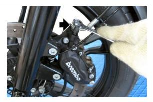
Remove the two calliper fixing screws
