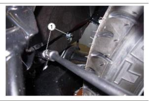
Remove the upper screws (2) taking care to recover the nuts
