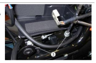
Move the filter box to the side enough to allow tightening of the fixing screws
