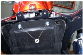
Remove the splash guard, pulling it to the rear
