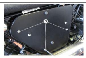
Remove the side fairing (4), recovering the three spacers (5) and the three washers (6).
