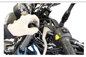
Disconnect the clutch cable from the disengagement lever
