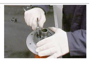
Remove the conical crown.
