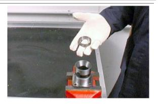
Slide off the tapered bearing from the case.
