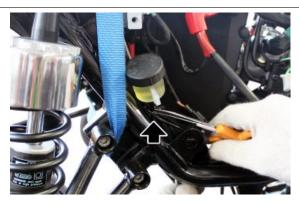
Remove the rear brake tank from the fork
