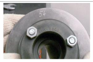
bearings on the bevel pinion holder case using the suitable punch (19926400).
