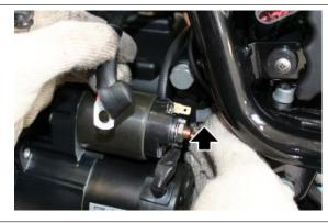
Remove the starter motor fixing screws
