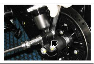
Remove the screw fixing the right-hand rear right shock absorber and pull it from the pin on the drive shaft
