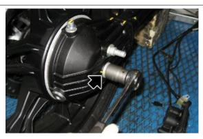
Loosen the wheel pin locking screw.
