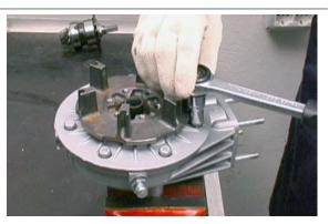
• When refitting the bevel pinion case on the transmission, bear in mind that the oil passage grooves with holes should be fitted vertically (observing the grooves, one should be facing upwards and the other facing the ground).
