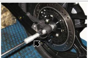
Remove the complete rear brake calliper support
