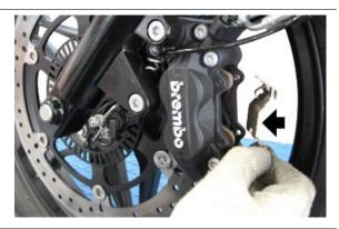
Remove the brake pads
