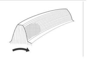
If the contact is like this, the pinion is too far from the rotation axis of the crown: approach the pinion by increasing spacer thickness
