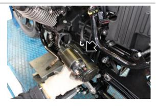
Remove the lambda probe, side stand and blow by recovery wiring retainer clamps
