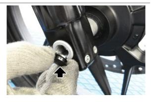
Loosen the two wheel pin locking screws;
