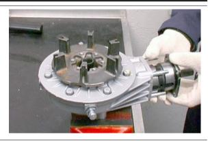
Lock on the vice the sealing tool (19907100) of the bevel gear pair.
