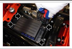
Remove sliding the complete filter box out toward the rear
