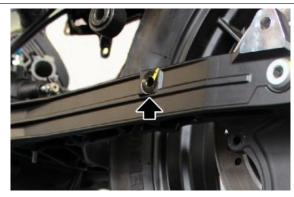
Remove the wheel pin and collect the spacer.
