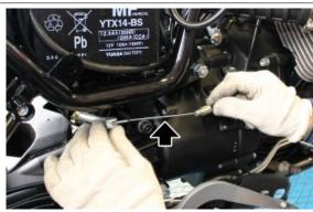
Remove the fixing screws of the right footrest support
