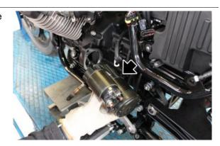
Disconnect the right Lambda probe connector and slide the cabling from the cable grommet
