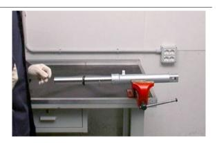
Screw the bottom screw and tighten it to the prescribed torque.
