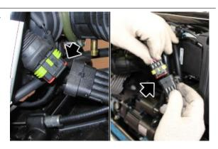
Unscrew and remove the two lambda probes.
