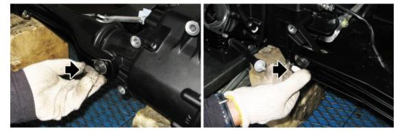
Loosen the pins so that the oscillating swingarm can be removed from the gearbox.
