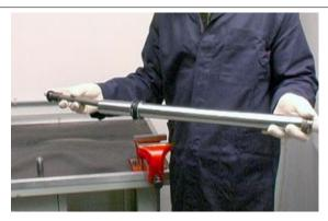
Check that the upper guide bushing is fitted on the wheel holder fork leg.
