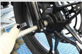
Working on the opposite side, remove the left spacer;
