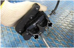
Remove the brake pads
