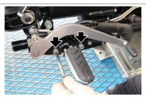
Remove the lower fixing pin of the cradle making sure to collect the washer and the nut
