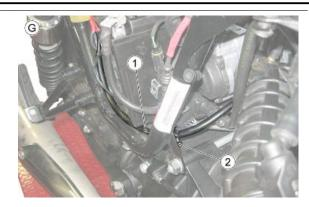
• Check that the hood which covers the starter motor positive is inserted well and that the nut is secured correctly to the prescribed torque.
