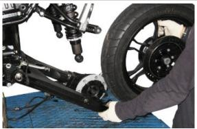
Working on the left side, remove the spacer;
