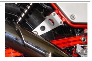
Fit the exhaust mounting plate preset for fixing the passenger footrest, so as to turn the vehicle into a two seater version.
