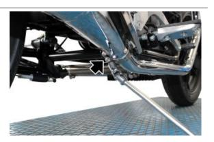
Unscrew and remove the muffler fixing nut and collect the screw and the bushing.
