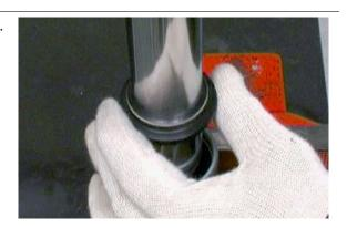
Remove the locking ring inside the fork leg using a thin screwdriver.
