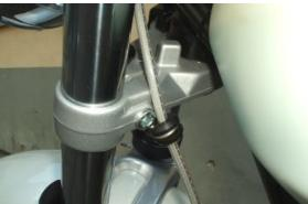
• Slide off the stem downwards by turning it slightly first in one direction then to the opposite direction.
