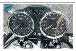
Working from both sides, undo and remove the screw locking the upper plate to the front fork.
