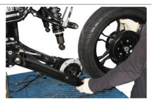
Cut the sealing clamp and lift the folding
