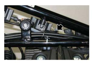
Disconnect the coil connector, turn the key to ON and activate the component through the diagnostics instrument.
