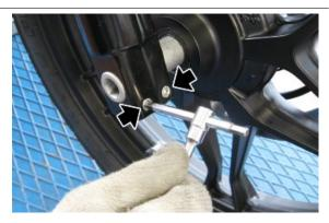
Unscrew and remove the wheel pin;
