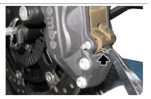
Remove the brake pad retaining pins
