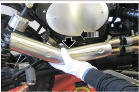
Disconnect the connectors of the lambda probes
