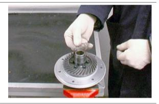
Fit the braking disc on the drilled bolt by locking the screws with the washers using a torque wrench.
