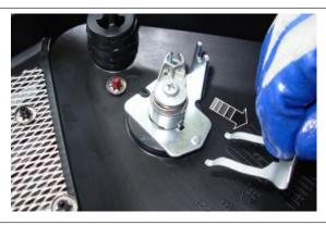
• Remove the cable support plate
