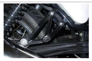
Fit the countersunk screw with hexagonal hole on "C" supporting the pedal and afterwards fit the washer.
