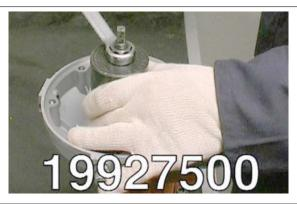
Remove the sealing ring and the washer.
