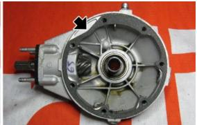
Remove the external ring of the needle bearing from the housing using the suitable extractor (19927500).
