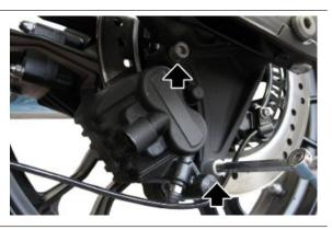
Remove the screws locking the brake pads
