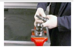
Fit the complete pinion on the case using the suitable punch (19926100).
