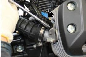
• Disconnect the engine temperature sensor connector
