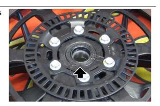
Using a generic bearing extractor remove the bearings from both sides
