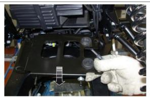
Unscrew the clamp that fastens the throttle body to the air filter box
