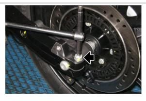
Unscrew and remove the fixing screw of the calliper holder.
