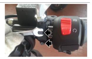
Remove the brake pump
