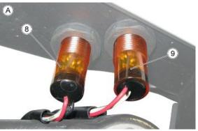
The wiring harness of the warning lights must pass in the points indicated in the figure.
