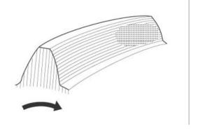
If the contact is like this, the crown is too far from the pinion rotation axis: approach the crown by reducing spacer thickness.
