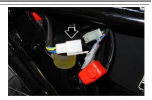
Remove the rear mudguard by sliding the light cabling through the wheel housing
